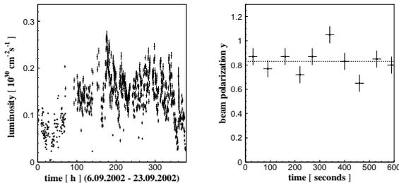
**Fig. 1:** (a) On-line determination of the luminosity during the September '02 measurements of  $\bar{p}p \rightarrow pp\eta$  reaction. (b) On-line estimation of the beam polarization as measured using the EDDA polarimeter – the value of vertical beam polarization is shown versus the time of the cycle.
