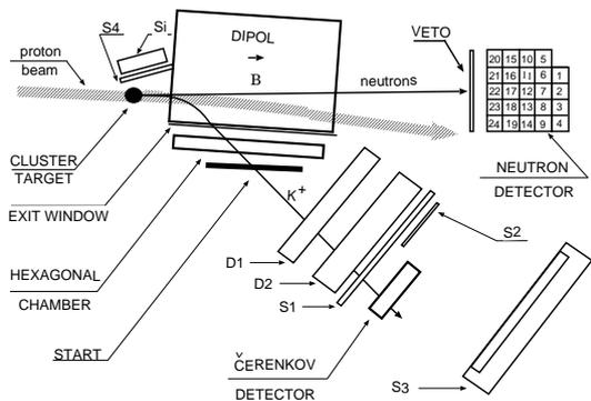
Fig. 2: COSY-11 setup with neutron detector [9] and additional kaon start scintillator to perform the measurement of the threshold  $\Sigma^+$  production.
