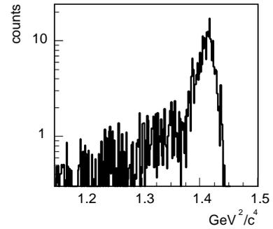
Fig. 3: Expected missing mass distribution for  $\Sigma^+$  generated with a realistic Monte Carlo study.
