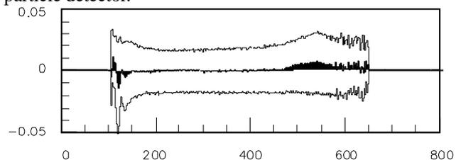
**Fig. 1:** Example of the spectrum used for the drift chamber calibration. Shaded area presents mean values of  $\Delta X$  (in cm) as a function of the drift time (in ns). Upper and lower histograms indicate a band of one standard deviation of the  $\Delta X$  distribution.
