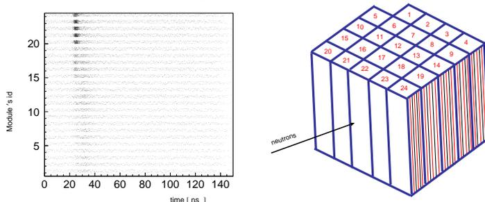
**Fig. 3:** (left) Time-of-flight determined between the target and the neutral particle detector as a function of module's number. (right) Configuration of the detection units
