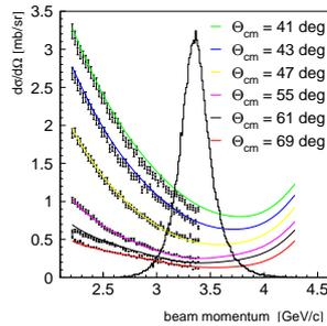
**Fig. 2:** Differential cross sections as a function of beam momentum for few values of a scattering angle in the center-of-mass system  $\theta_{cm}$ . Black points stand for EDDA collaboration data [3], lines denote SAID calculations [4]. The solid histogram denotes the distribution of the effective beam momentum for quasi-free  $pp \rightarrow pp$  reaction calculated at the beam momentum of 3.35 GeV/c.
